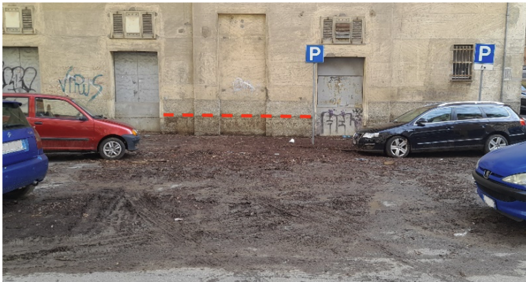
Figure 4. Pictures showing post-event traces of the ground effects of the event analysed. The red dashed line shows traces of the water level reached during the event.
