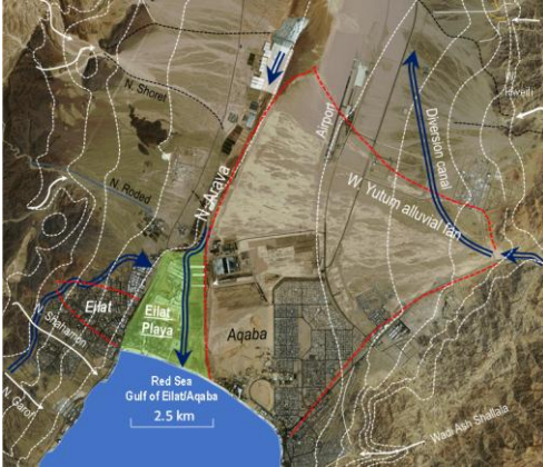
Figure 56: Visible active distributary channels on the Wadi Yutum alluvial fan. Since the picture was taken (2004), the city has grown without leaving short flowpath to the sea; instead, several retention dams are constructed to reduce sediments and diversion canal to bypass the city (Eom et al., 2011). The canal increases the flow path to the Red Sea from 8.5 to 27 km (slope drop from 2.4 to 0.7 % respectively), reducing sediments carrying capacity of flood. Source: ©Google Earth 2004.
