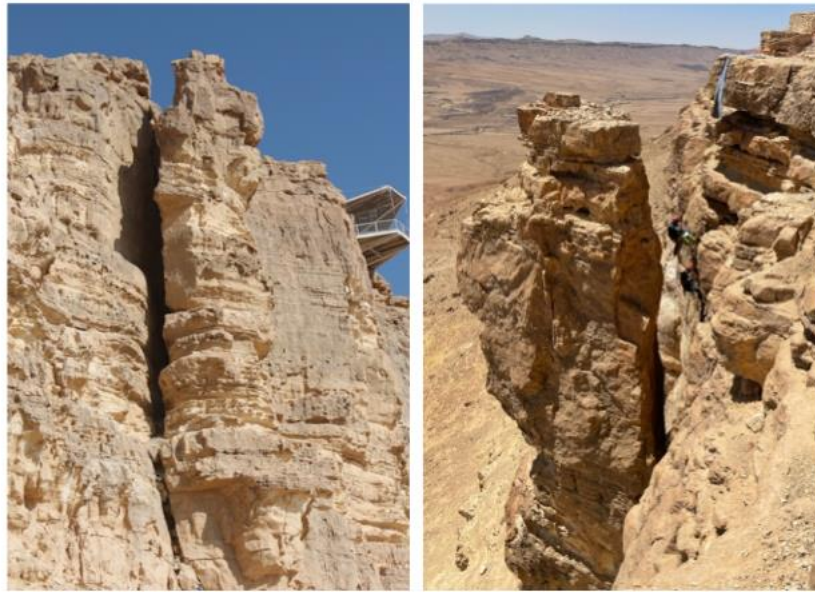
Figure 2. The Ramon pillar: a) photo taken from the Ramon crater floor, looking northeast (left); b) rappelling along the back crack for measurement of rock elastic modulus, looking southwest (right).
