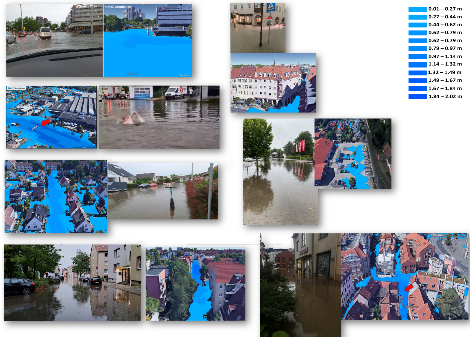
Figure B1. Examples of comparisons between the dx = 5 m RIM2D simulation results to social media posts. Visualization of the RIM2D results and the background imagery are performed with and provided by Google Earth. Satellite imagery: Google Earth 2024
