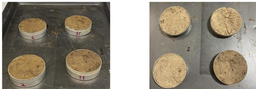
435 (a) Wet undisturbed cylinder samples A (b) Undisturbed cylinder samples A after being dried
