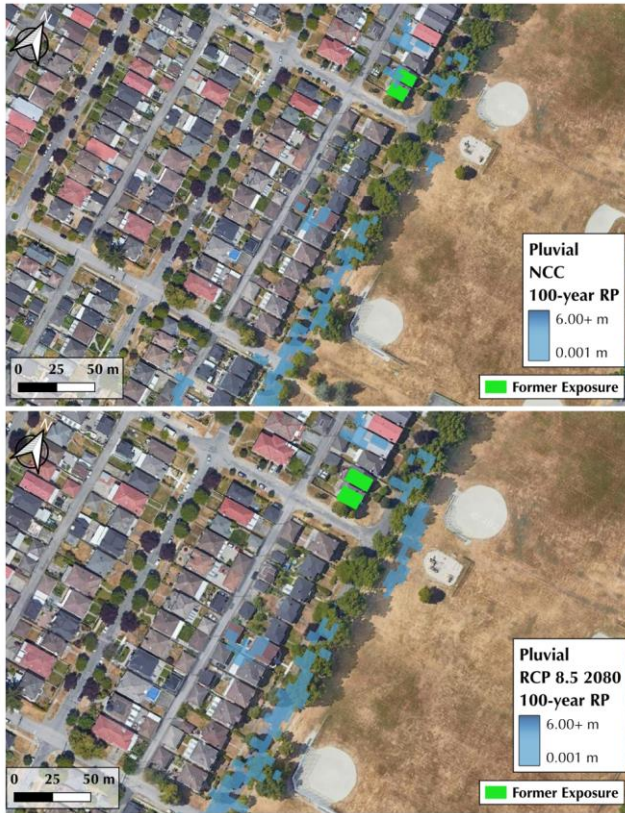
Figure 6: Example of Two Assets Considered Exposed at the NCC State and not at RCP 8.5 2080 Climate State. Other map data: Google Satellite Imagery ©2023, CNES / Airbus, Maxar Technologies ©2023
