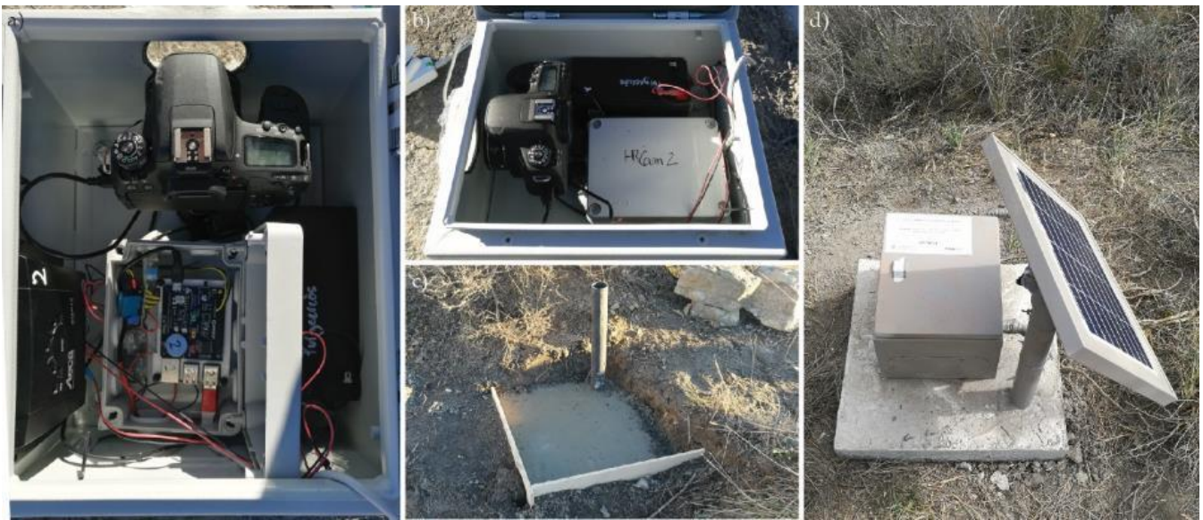
Figure 1. Images of the photogrammetric systems installed in the Puigcercós site: a and b) Images showing the inside of the photogrammetric unit with part of the connections shown in Figure 3; c) Construction of the concrete base and installation of the PVC pipe for the installation of the photographic units and d) external view of the installed system.
