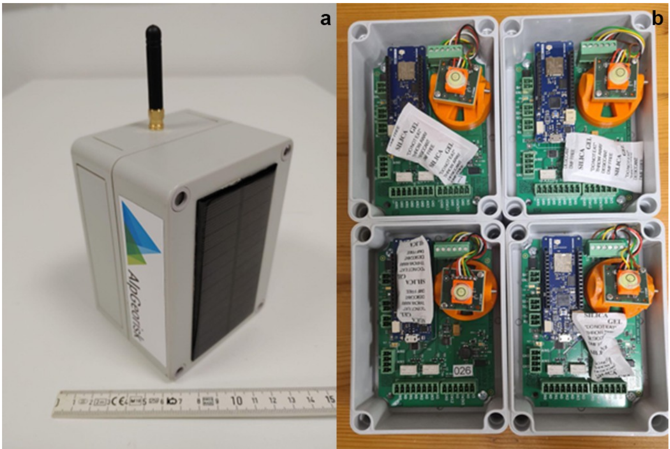
Figure 9. (a) Sensor Node with mounted solar panel for autarkic operation (b) Inside view on four sensor nodes. The Arduino microprocessor MKR WAN 1310 (blue PCB) is connected to the Inform@Risk sensor PCB (large green PCB), which contains a suite of different sensors including a thermometer, barometer, 4-channel 24 bit ADC and an accurate tiltmeter, which is mounted on an orange rotatable base to make leveling of the sensor independent of the box orientation possible.
