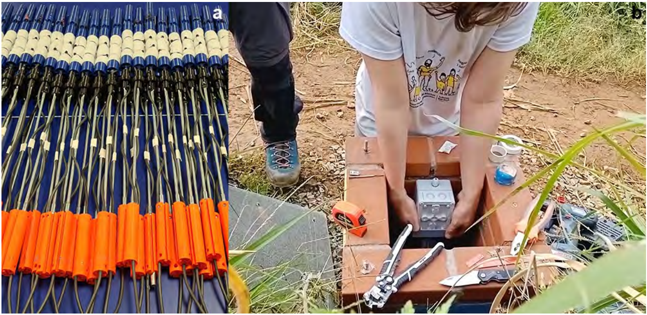
355 Figure 10. (a) Sensor Probes ready for installation. The piezometer (blue) is located at the bottom of the probe. Above follows a ball joint (black) which exactly fits into the used installation pipes and functions as reference points for the inclination measurements. Above follows the first inclination sensor (orange), which - when installed - is followed by another ball joint (2nd reference point located exactly 1 m above first joint). If required, further inclination sensors can be added. (b) installation of subsurface probe into a brick seating cube.
