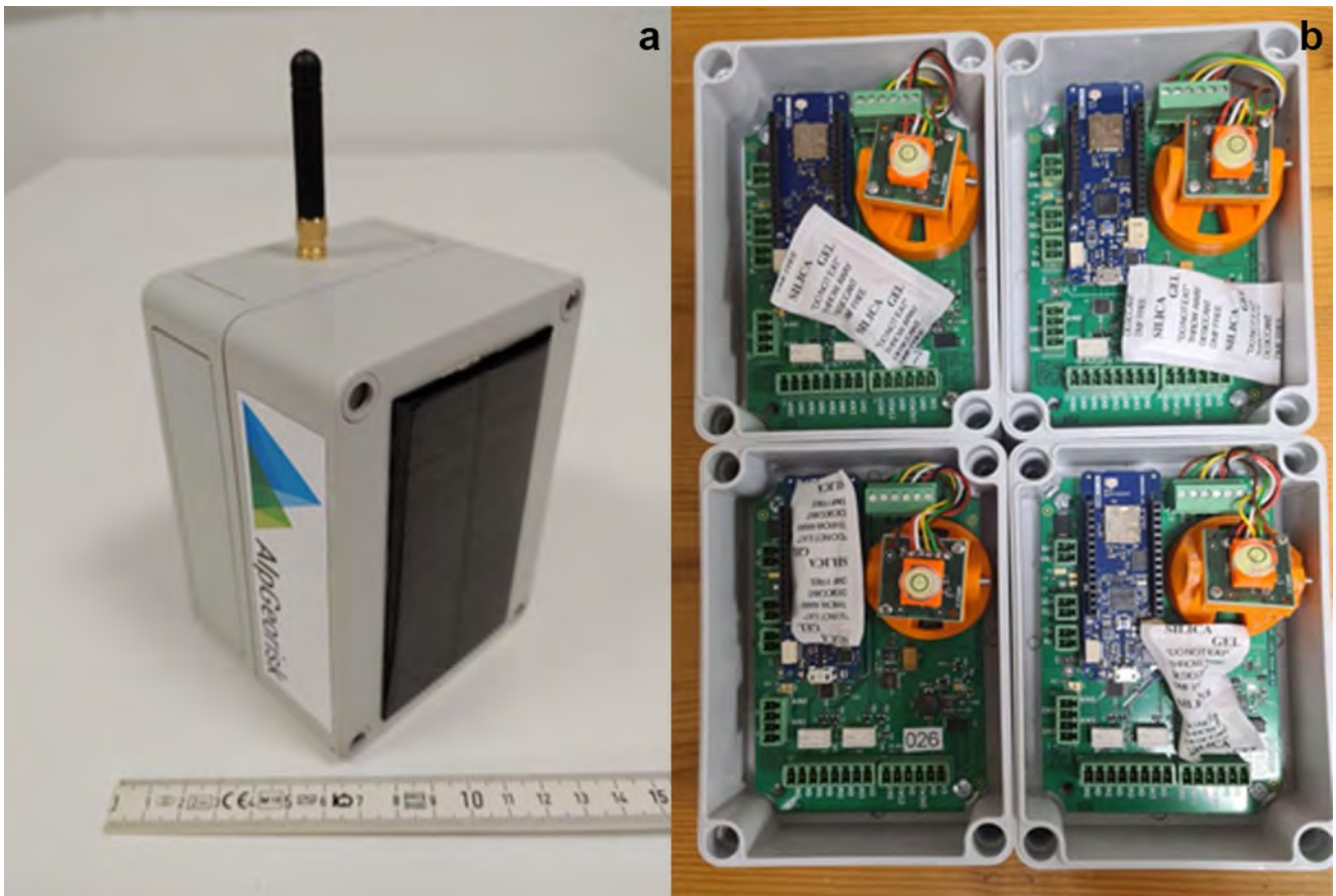
345 Figure 9. (a) Sensor Node with mounted solar panel for autarkic operation (b) Inside view on four sensor nodes. The Arduino microprocessor MKR WAN 1310 (blue PCB) is connected to the Inform@Risk sensor PCB (large green PCB), which contains a suite of different sensors including a thermometer, barometer, 4-channel 24 bit ADC and an accurate tiltmeter, which is mounted on an orange rotatable base to make leveling of the sensor independent of the box orientation possible.
