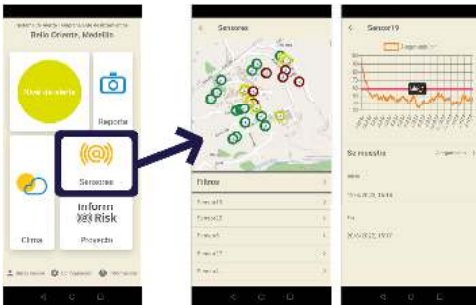
Figure A4. Interfaces of the warning app (from left to right): main menu of the App, map of sensor distribution, and information provided by sensor.
