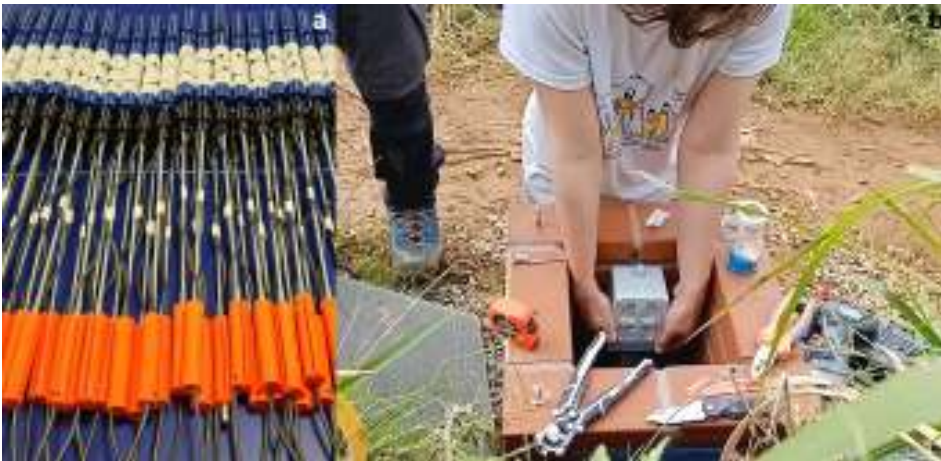
370 Figure 10. (a) Sensor Probes ready for installation. The piezometer (blue) is located at the bottom of the probe. Above follows a ball joint (black) which exactly fits into the used installation pipes and functions as reference points for the inclination measurements. Above follows the first inclination sensor (orange), which - when installed - is followed by another ball joint (2nd reference point located exactly 1 m above first joint). If required, further inclination sensors can be added. (b) installation of subsurface probe into a brick seating cube.
