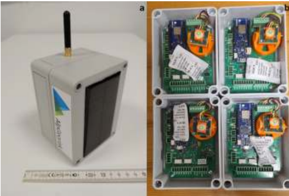
360 Figure 9. (a) Sensor Node with mounted solar panel for antarctic operation (b) Inside view on four sensor nodes. The Arduino microprocessor MKR WAN 1310 (blue PCB) is connected to the Inform@Risk sensor PCB (large green PCB), which contains a suite of different sensors including a thermometer, barometer, 4-channel 24 bit ADC and an accurate tiltmeter, which is mounted on an orange rotatable base to make leveling of the sensor independent of the box orientation possible.
