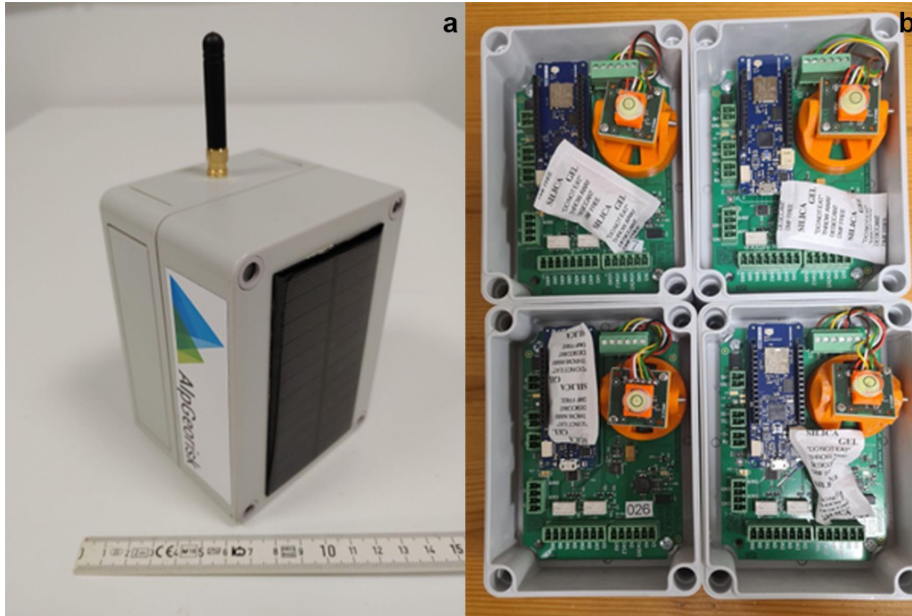
Figure 9. (a) Sensor Node with mounted solar panel for autarkic operation (b) Inside view on four sensor nodes. The Arduino microprocessor MKR WAN 1310 (blue PCB) is connected to the Inform@Risk sensor PCB (large green PCB), which contains a suite of different sensors including a thermometer, barometer, 4-channel 24 bit ADC and an accurate tiltmeter, which is mounted on an orange rotatable base to make leveling of the sensor independent of the box orientation possible.
