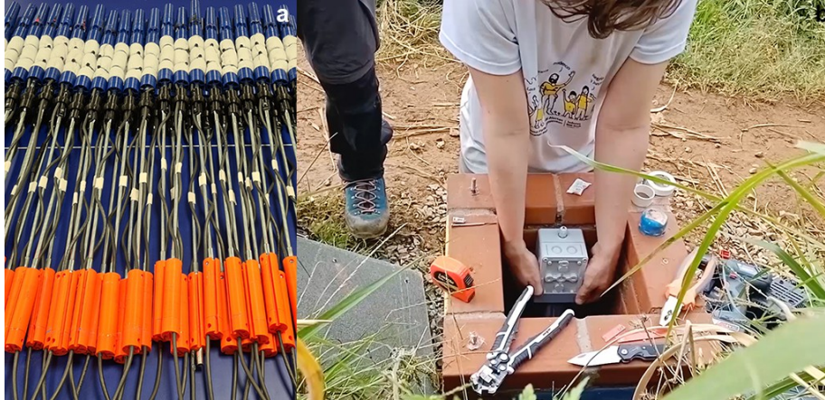
Figure 10. (a) Sensor Probes ready for installation. The piezometer (blue) is located at the bottom of the probe. Above follows a ball joint (black) which exactly fits into the used installation pipes and functions as reference points for the inclination measurements. Above follows the first inclination sensor (orange), which - when installed - is followed by another ball joint (2nd reference point located exactly 1 m above first joint). If required, further inclination sensors can be added. (b) installation of subsurface probe into a brick seating cube.
