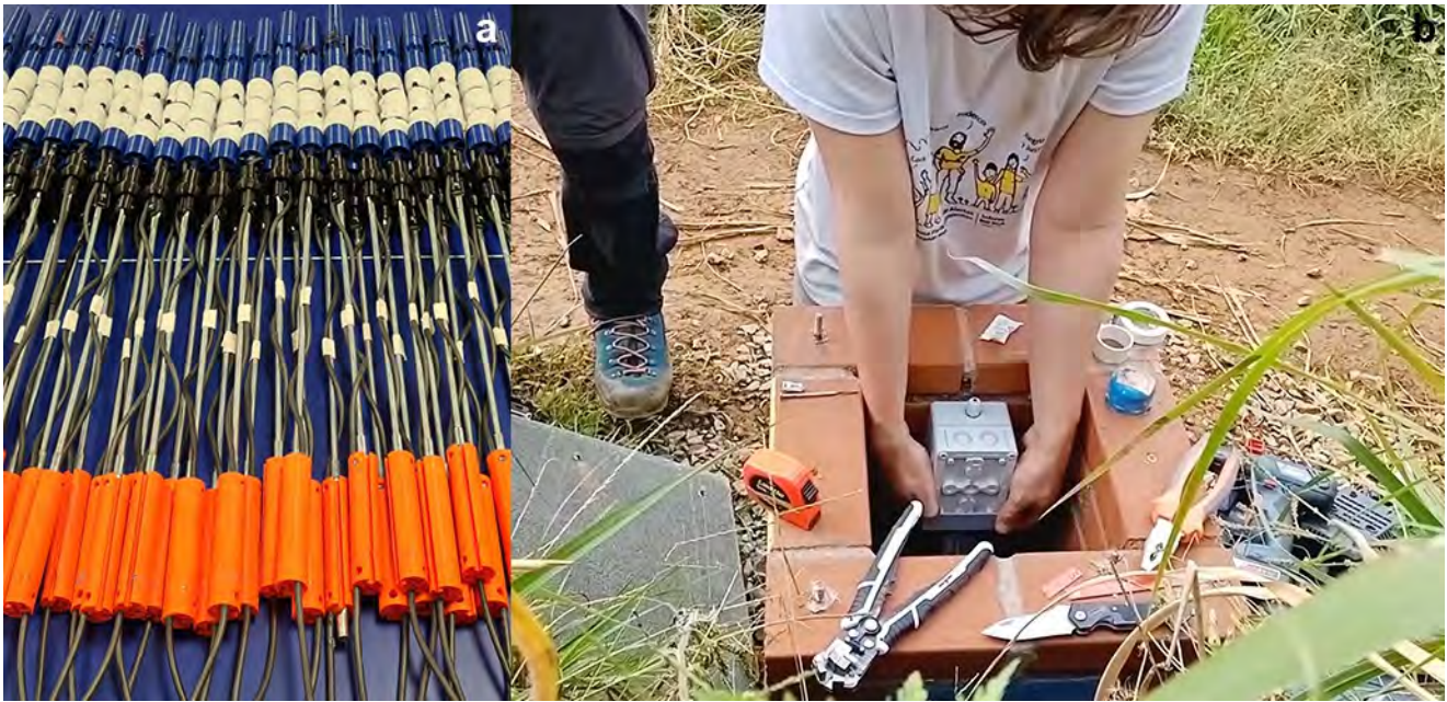
365 Figure 10. (a) Sensor Probes ready for installation. The piezometer (blue) is located at the bottom of the probe. Above follows a ball joint (black) which exactly fits into the used installation pipes and functions as reference points for the inclination measurements. Above follows the first inclination sensor (orange), which - when installed - is followed by another ball joint (2nd reference point located exactly 1 m above first joint). If required, further inclination sensors can be added. (b) installation of subsurface probe into a brick seating cube.
