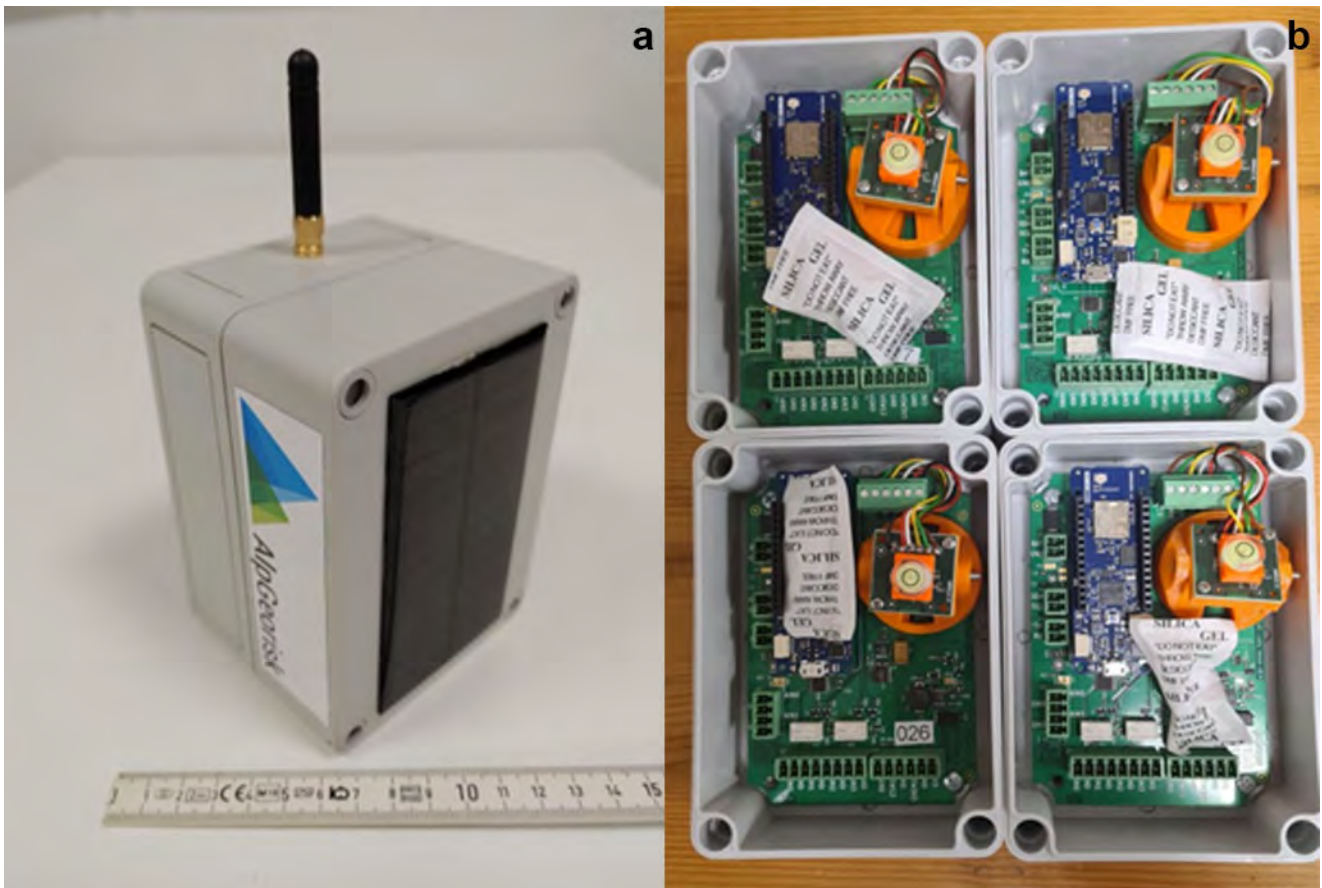
355 Figure 9. (a) Sensor Node with mounted solar panel for autarkic operation (b) Inside view on four sensor nodes. The Arduino microprocessor MKR WAN 1310 (blue PCB) is connected to the Inform@Risk sensor PCB (large green PCB), which contains a suite of different sensors including a thermometer, barometer, 4-channel 24 bit ADC and an accurate tiltmeter, which is mounted on an orange rotatable base to make leveling of the sensor independent of the box orientation possible.
