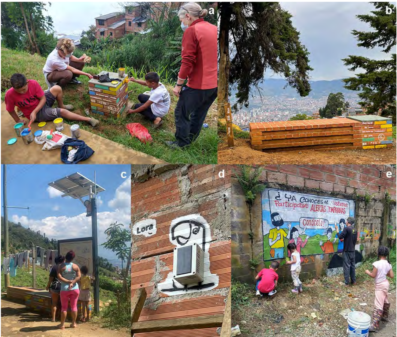
435 Figure 12. (a) Collaborative painting of a brick seating cube with a subsurface probe inside (b) a micro garden next to a brick bench sheltering a Subsurface Probe (c) Brick bench housing the central monitoring station and an information board (d) Inclinometer sensor on a private home with the Inform@Risk mascot “Lora” (e) murals painted by local artists with the help of children.
