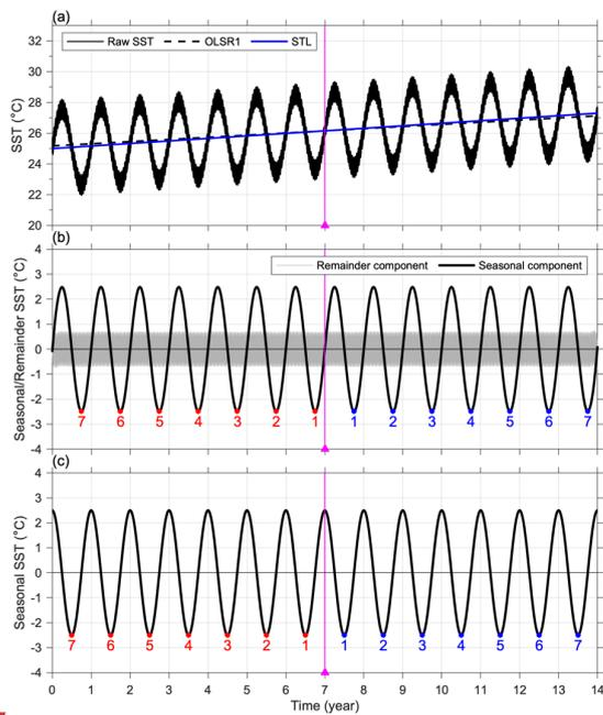
Figure 5: (a) Time series of simulated SST using (1) and (3) and its regressions using OLSR1 and STL, (b) seasonal and remainder components derived from STL, and (c) the seasonal variations using the cosine function shown as (4). The numbers in (b) and (c) denote the corresponding seasonal peaks on the two sides of the mid-time (magenta lines).
