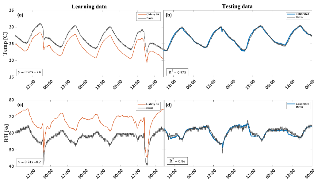
135 Figure 2. Temperature and RH control experiment with a stationary smartphone (Samsung Galaxy S4) and an adjacent weather station (Davis Vantage VUE), conducted in Israel. (a) & (c) Raw smartphones (red) and weather station (black) T & RH values, respectively, during 4 days (2-6 October). (b) & (d) Smartphone calibrated data (blue) and weather station (black) T & RH values respectively for a different 4 days (7-10 October).
