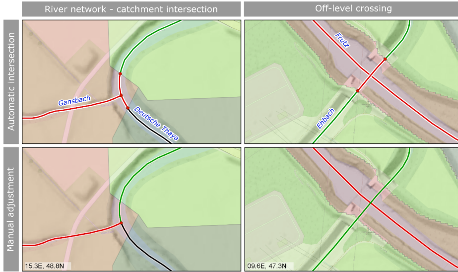
210 Figure 3: Automatic (upper row) and manual (lower row) procedures to associate the catchment boundaries with the river network. Left: Merging of the two outer red nodes that arise from position accuracies of the catchment boundary of the Gansbach, tributary to the Deutsche Thaya, Lower Austria. Right: Ehbach crossing under the Frutz in Vorarlberg. The river reach and associated catchment area have matching colours.
