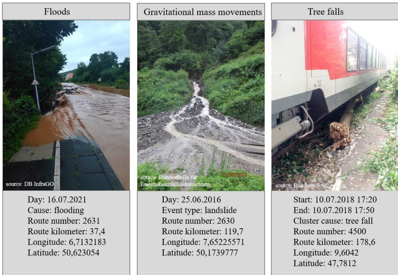
Figure 3: Examples of recorded events for all three types of natural hazards in the damage database of DB InfraGO. Note that the level of detail is different for the different type of events. For floods and gravitational mass movements, the fields “cause” and “event type” are free text fields, while for tree falls the two options “tree fall” and “branch breakage” can be selected in the field “cluster cause”.
