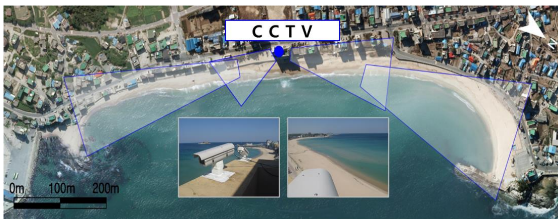
Figure 14: Video monitoring using four CCTVs at Bongpo-Cheonjin Beach (MOF, 2019; © National Geographic Information Institute (NGII), Korea).
