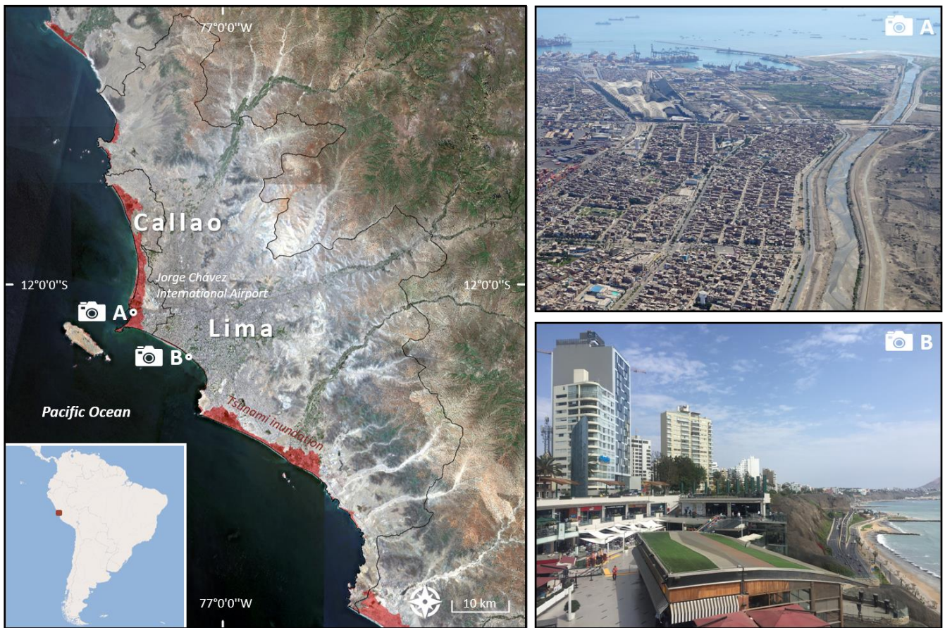
375 Figure 4. Multispectral satellite image (left) of the study area of Lima Metropolitan area, Peru, with administrative boundaries (black outlines). Additionally, an estimated tsunami inundation exemplified for a Mw 8.9 earthquake (generated with TsunAWI; Harig et al., 2008) is shown. Coastal features such as the harbour in Callao (upper right) and the coastal highway in Miraflores (lower right) are displayed. Photographs taken by (A) Torsten Riedlinger (2018) and (B) Elisabeth Schoepfer (2019). Map data © Copernicus Sentinel data 2023, processed by ESA; © DLR, EOC Basemap Map Service 2023; © Instituto Geográfico Nacional, Limites Distritales 2022.
