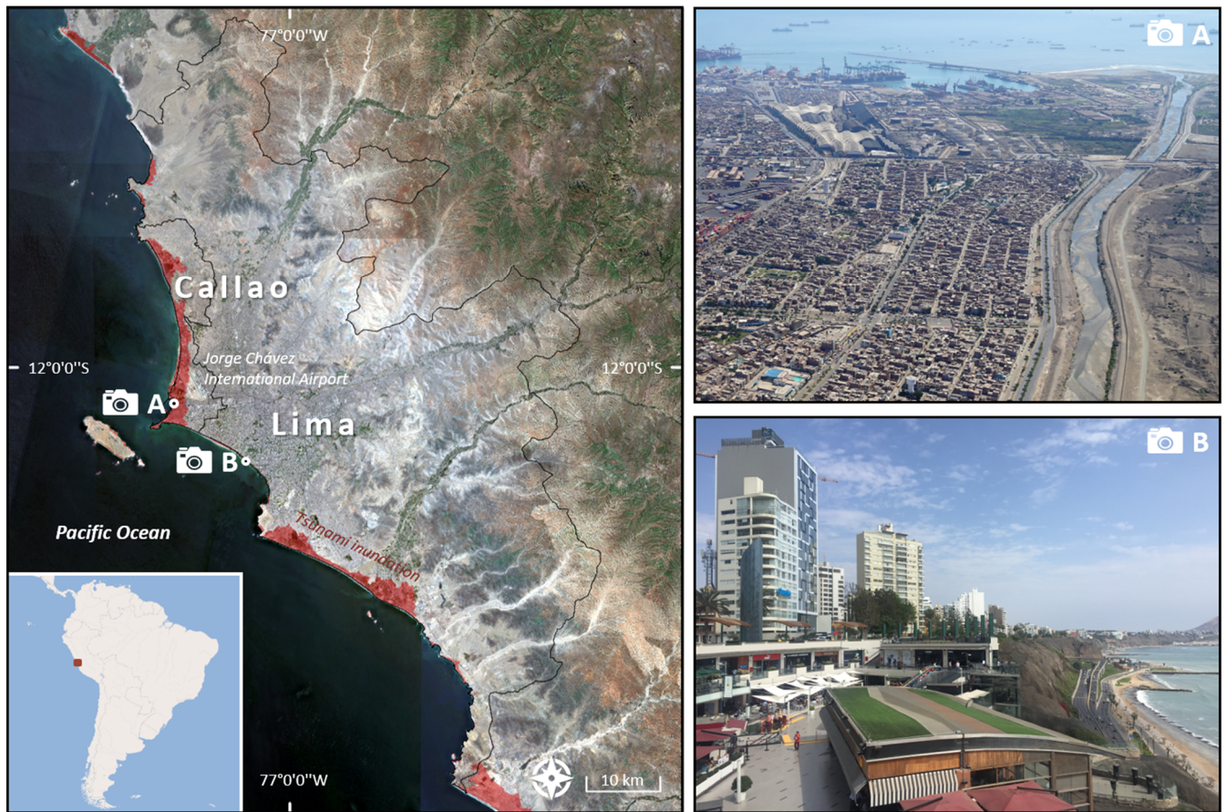
395 Figure 4. Multispectral satellite image (left) of the study area of Lima Metropolitan area, Peru, with administrative boundaries (black outlines). Additionally, an estimated tsunami inundation exemplified for a Mw 8.9 earthquake (generated with TsunAWI; Harig et al., 2008) is shown. Coastal features such as the harbour in Callao (upper right) and the coastal highway in Miraflores (lower right) are displayed. Photographs taken by (A) Torsten Riedlinger (2018) and (B) Elisabeth Schoepfer (2019). Map data © Copernicus Sentinel data 2023, processed by ESA; © DLR, EOC Basemap Map Service 2023; © Instituto Geográfico Nacional, Limites Distritales 2022.
