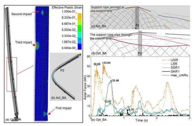
Figure 17: Opt\_BA calculation result: (a) The column P2 in Opt\_BA got local damages after several hits. (b) The column P2 in Act\_BA was buckling. (c) and (d) are the support rope sliding performance on the end of column P3 in Act\_BA and Opt\_BA, respectively, where semi-transparent for pre-impact and saturated color for post-impact. (e) The internal force of part of the wire ropes in Opt\_BA.
