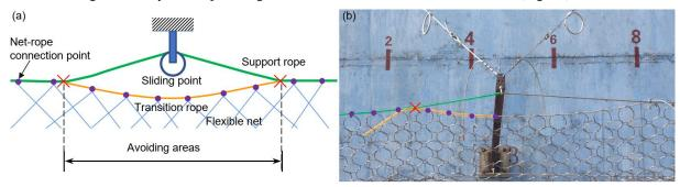
Figure 13: The transition rope applied between column ends and support ropes: (a) Structure schematic and (b) project photo.
