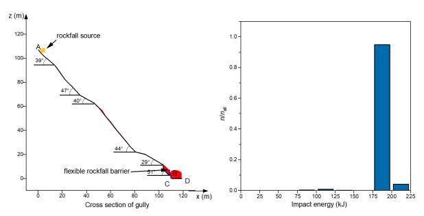
Figure 7: Rockfall movement analysis: (a) Trajectory of rockfall and (b) Probability distribution of kinetic energy of falling rocks at the flexible barrier.
