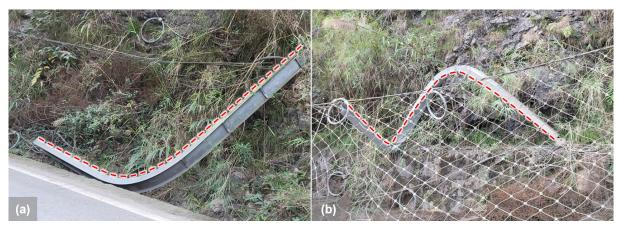
Figure 2: Steel column buckling forms of the other two flexible rockfall barrier projects: (a) "C"-shaped compression buckling and (b) "S"-shaped bending and torsion buckling.
