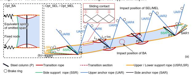
Figure 14: Structure representation of the model Opt\_. (a) Simulation models Opt\_SEL and Opt\_MEL. (b) Simulation model Opt\_BA.
