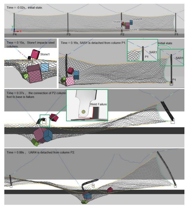
Figure 8: Keyframes of the impact process (the 0 instant occurs when Stone3 touches the wire rope net).
