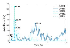
Figure 10: Axial force of the Wire ropes in Act\_BA
