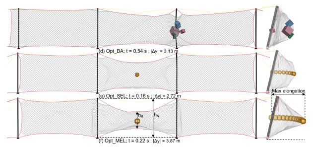
Figure 15: System forms at the moment of maximum y-directional deformation.
