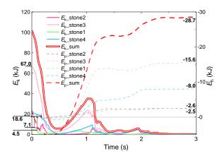
Figure 11: Temporal evolution of kinetic energy and potential energy of rockfalls.
