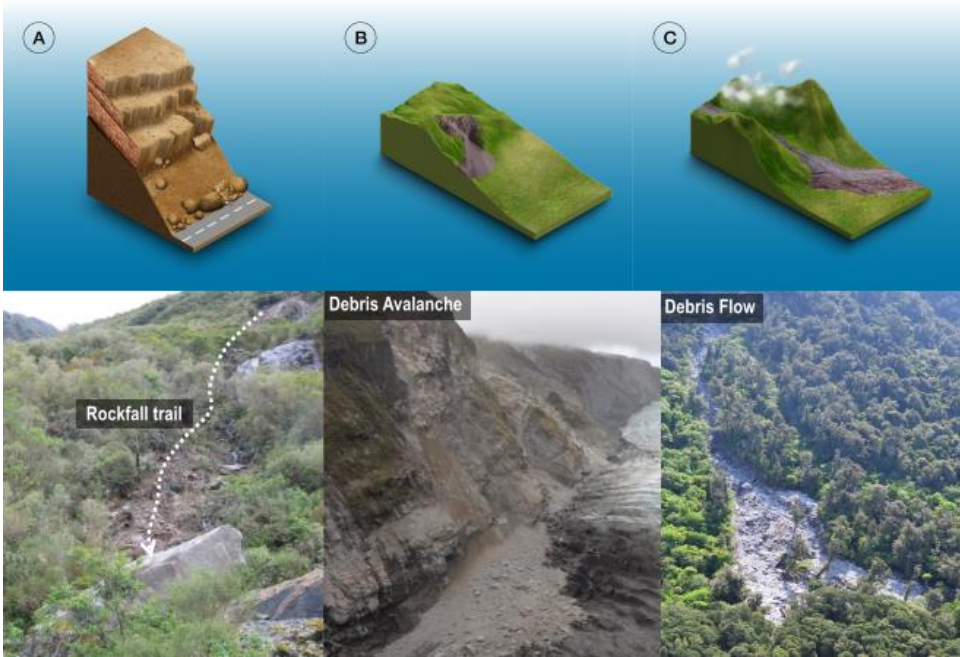
115 Figure 2: Schematic and example photographs of landslide types considered in the ORA, including a) rockfall, b) debris and rock avalanches, and c) debris flows.
