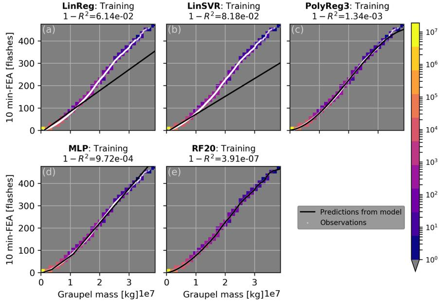
**Figure 6.** Model training curves in black for (a) linear regression, (b) linear support vector machine, (c) cubic polynomial regression, (d) multi-layer perceptron and (e) random forest regression overlaid on the global sorted distribution of observed FEA versus simulated graupel mass in white. The colour shades represent the number of points in each bin of  $0.13 \times 10^7$  kg width.
