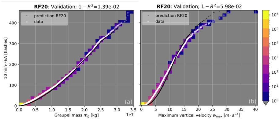
**Figure 8.** Sorted distribution for the validation set of the observed FEA versus the simulated graupel mass (a) and maximum vertical velocity (b) in white. Black dots correspond to the FEA predicted by the RF20 regression.
