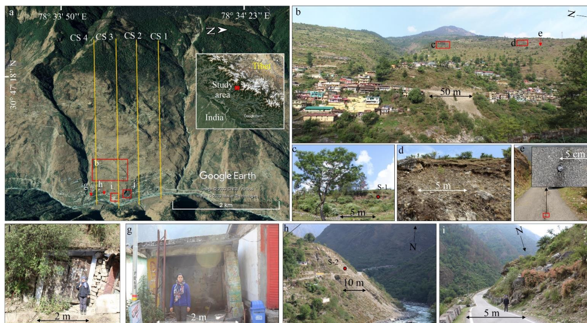
8 Fig. 2. Field observation of Bhatwari town. (a-b) Location of Bhatwari town with inset highlighting the 9 position in the NW Himalaya. CS 1 to CS 4 mark the position of 2D slope sections used for the slope 10 stability evaluation; (c-d) Exposed scarp. S-1 refers to soil sampling site; (e) Cracks and displacement of 11 road; (f-g) Tilting houses/shops; (h) Active slope failure at slope toe; (i) Big Gneissic boulder implying 12 paleo-landslide site.
