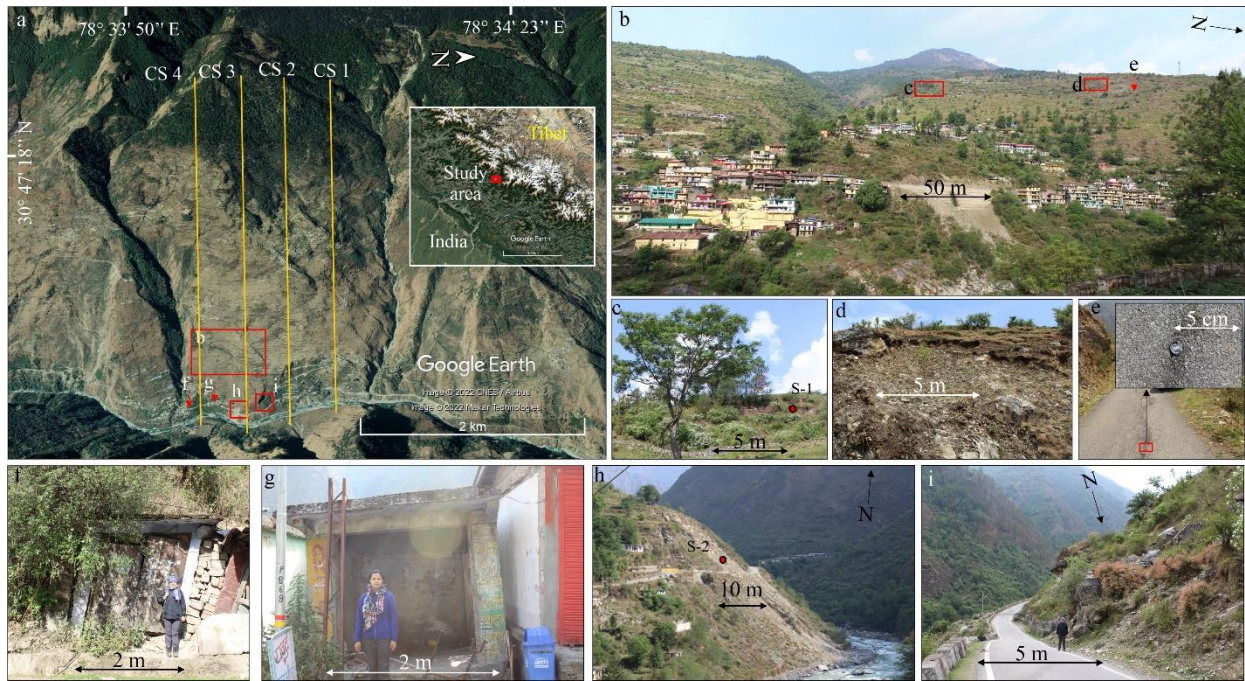
Fig. 2. Field observation of Bhatwari town. (a-b) Location of Bhatwari town with inset highlighting the position in the NW Himalaya. CS 1 to CS 4 mark the position of 2D slope sections used for the slope stability evaluation; (c-d) Exposed scarp. S-1 refers to soil sampling site; (e) Cracks and displacement of road; (f-g) Tilting houses/shops; (h) Active slope failure at slope toe; (i) Big Gneissic boulder implying paleo-landslide site.
