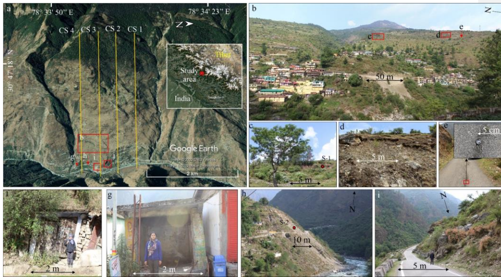
9 Fig. 2. Field observation of Bhatwari town. (a-b) Location of Bhatwari town with inset highlighting the 10 position in the NW Himalaya. CS 1 to CS 4 mark the position of 2D slope sections used for the slope 11 stability evaluation; (c-d) Exposed scarp. S-1 refers to soil sampling site; (e) Cracks and displacement of 12 road; (f-g) Tilting houses/shops; (h) Active slope failure at slope toe; (i) Big Gneissic boulder implying 13 paleo-landslide site.
