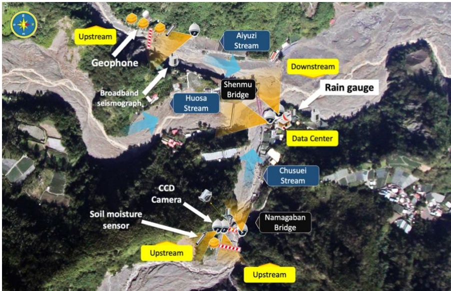
Figure 2: The layout of sensors installed at the Shenmu monitoring station. (base map credit: GIS Research Center, Feng Chia University, Taiwan).
