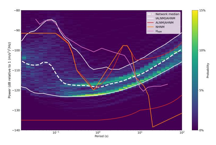
Figure 3. PSD probability density function of RAN. Dashed white line represents the median of the network and dotted lines are the 5% and 95% limits of the network. Solid green lines represent the ALNM and AHNM defined by Cauzzi and Clinton (2013). Red, and purple lines are NHNM and  $H_{INM}$  defined by Peterson (1993) and D'Alessandro et al. (2021), respectively.
