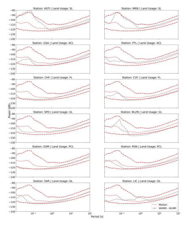
**Figure 5.** Median PSD of 2 randomly selected stations from each land usage type defined in Table 1. Red dashed line and dots represent the median and IAHNM&IAHNM, respectively.
