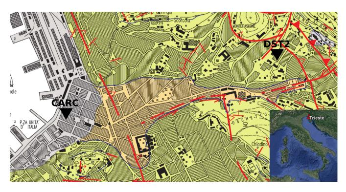
**Figure 10.** Geological Map of Trieste (grey, orange, and yellow colors indicate anthropic, ubiquitous deposit units, and flysh of Trieste, respectively), modified from Cucchi et al. (2013). Map on the lower right is created by using © Google Earth with satellite information from Landsat/Copernicus.
