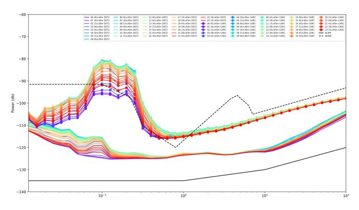
**Figure 11.** Hourly average plots of noise levels of DST2 (line) and CARC (line with dots). ALNM and AHNM introduced by Cauzzi and Clinton (2013) are black line and dashed line, respectively.
