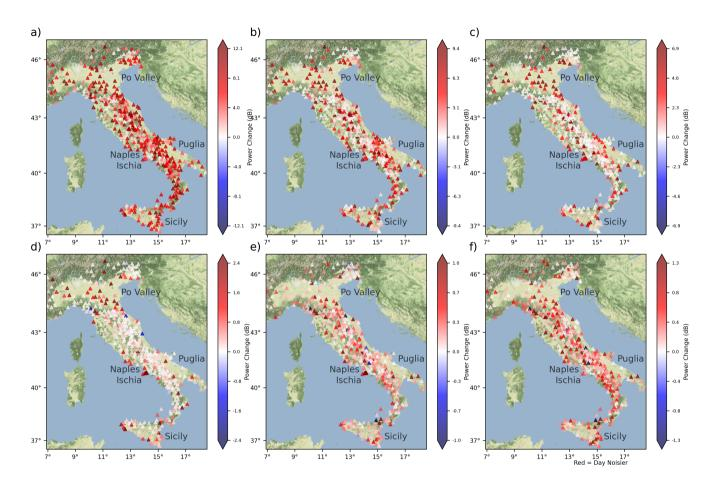
Figure 7. Difference between daytime and nighttime for the periods of a)  $0.1 \, \mathrm{s}$ , b)  $0.25 \, \mathrm{s}$ , c)  $0.5 \, \mathrm{s}$ , d)  $1.0 \, \mathrm{s}$ , e)  $2.0 \, \mathrm{s}$ , and f)  $5.0 \, \mathrm{s}$  in dB. Red color means day is noisier than night. Basemap data are retrieved from © Stamen Design.
