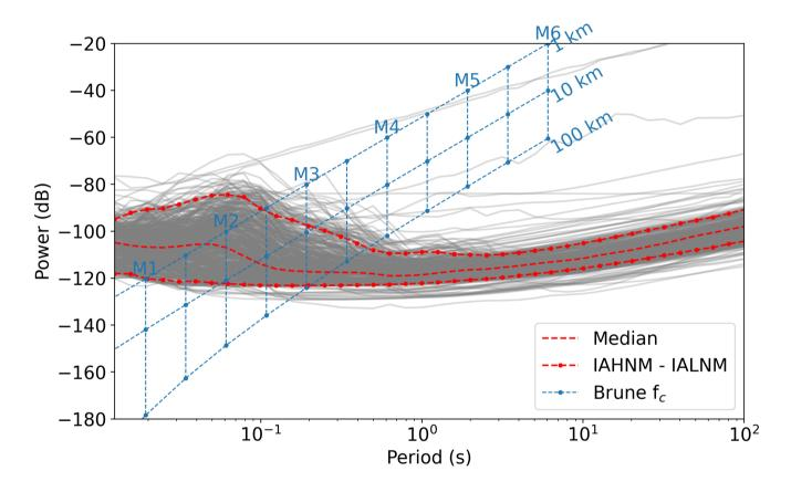
Figure 4. Median PSD of RAN stations (grey lines). Red dashed line and dots represent the median and IAHNM&IAHNM, respectively.
