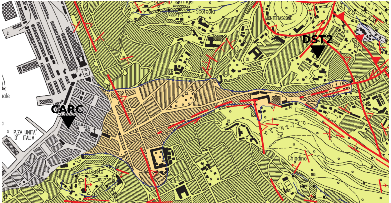
Figure 11. Geological Map of Trieste (grey, orange, and yellow colors indicate anthropic, ubiquitous deposit units, and flysch of Trieste, respectively), modified from Cucchi et al. (2013).
