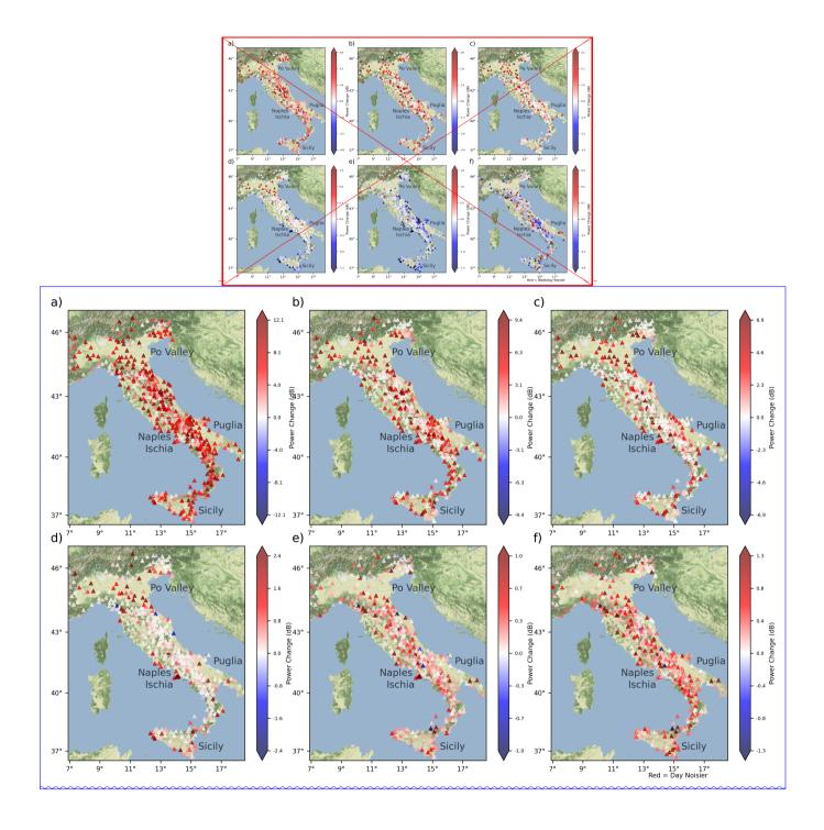
Figure 7. Median noise levels in dB for weekday Difference between daytime and weekend time nighttime for the periods of a) 0.1 s, b) 0.25 s, c) 0.5 s, d) 1.0 s, e) 2.0 s, and f) 5.0 s in dB. Red color means weekday day is noisier than weekendnight. Basemap data are retrieved from © Stamen Design.
