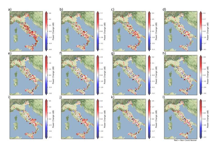
**Figure 10.** Difference between noise levels in  $0.1 \, \mathrm{s}$ ,  $0.25 \, \mathrm{s}$ ,  $0.5 \, \mathrm{s}$ ,  $1.0 \, \mathrm{s}$ ,  $2.0 \, \mathrm{s}$ , and  $5.0 \, \mathrm{s}$  between 2019 - 2022 and lockdown in a, c, e, g, i, k) daytime, b, d, f, h, j,l) nighttime. Basemap data are retrieved from © Stames Design.
