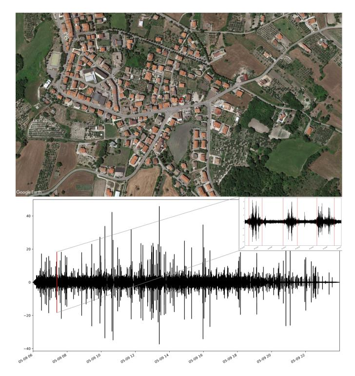
Figure 14. top) Satellite image of the Palata. PLTA station is demonstrated with (red triangle (, latitude: 41.88, longitude: 14.78) station which is located in Palata municipality building in Central Italy (the image is generated by © Google Earth). bottom). Seismic record registered on 9th of May 2019. Three detected cars are presented in the upper right with red vertical lines presenting the initiation and termination position of the car signals.
