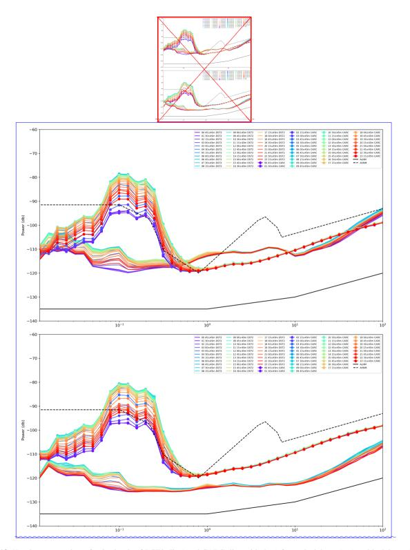
Figure 13. Hourly average plots of noise levels of DST2 (line) and CARC (line with dots) for no-lockdown (top) and lockdown (bottom) dates. ALNM and AHNM introduced by Cauzzi and Clinton (2013) are black line and dashed line, respectively.
