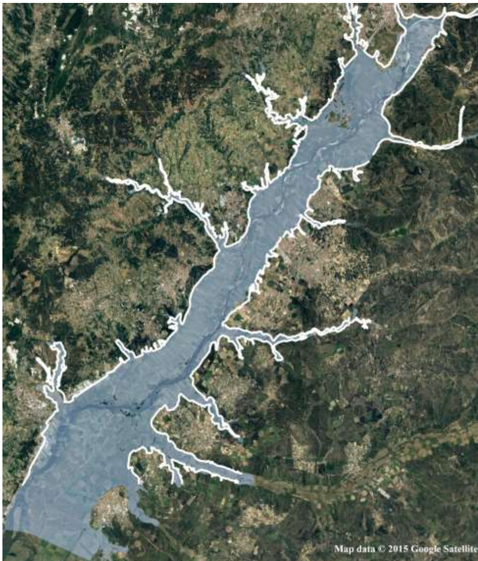
Figure 6. Maximum flood extension for event of February, 1979, in lower Tagus, obtained from the hydraulic simulation (Simulation_Control_1979). The white line represents the real extension of the flood reconstructed by the National Civil 890 Engineering Laboratory (LNEC) and the Water Institute (INAG) from Portugal ( www.snirh.pt ). Map data © Google Satellite.
