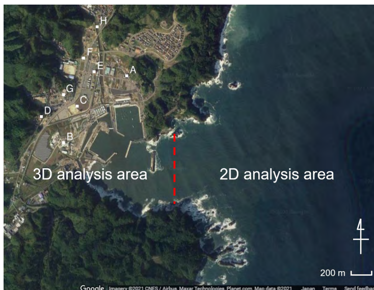
Figure 4. Boundary between 2D and 3D analyses areas. Points A to H are used to compare the inundation depths between the observational data and simulation results. (©Google Maps, Tozato et al. (2022) )
