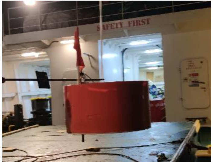
Figure 5 | DUNE OBS. New broadband OBS developed and build in Portugal with the new seismic sensor Aquarius (120s-100Hz) from GURALP and a broadband hydrophone HTI-04-PCA. On the left DUNE OBS on free-fall in the water column. On the right: Recovery of the DUNE OBS with the flag, radio and flashlight outside the orange shell. The deployment and recovery on board Portuguese vessel, RV Mário Ruivo (IPMA).
