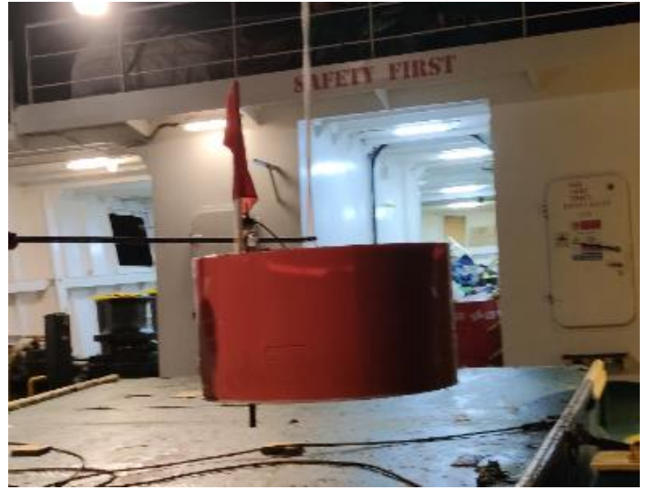
710 Figure 5 | DUNE OBS. New broadband OBS developed and build in Portugal with the new seismic sensor Aquarius (120s-100Hz) from GURALP and a broadband hydrophone HTI-04-PCA. On the left DUNE OBS on free-fall in the water column. On the right: Recovery of the DUNE OBS with the flag, radio and flashlight outside the orange shell. The deployment and recovery on board Portuguese vessel, RV Mário Ruivo (IPMA).
