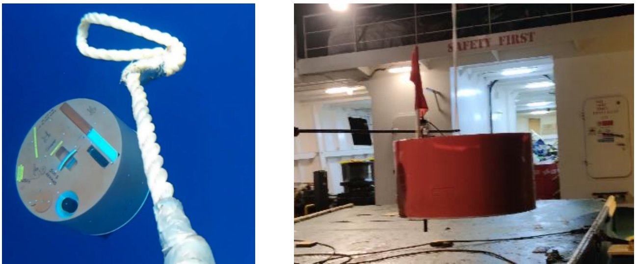
Figure 4 | DUNE OBS. New broadband OBS developed and build in Portugal with the new seismic sensor Aquarius (120s-100Hz) from GURALP and a broadband hydrophone HTI-04-PCA. On the left DUNE OBS on free-fall in the water column. On the right: Recovery of the DUNE OBS with the flag, radio and flashlight outside the orange shell. The deployment and recovery on board Portuguese vessel, RV Mário Ruivo (IPMA).
