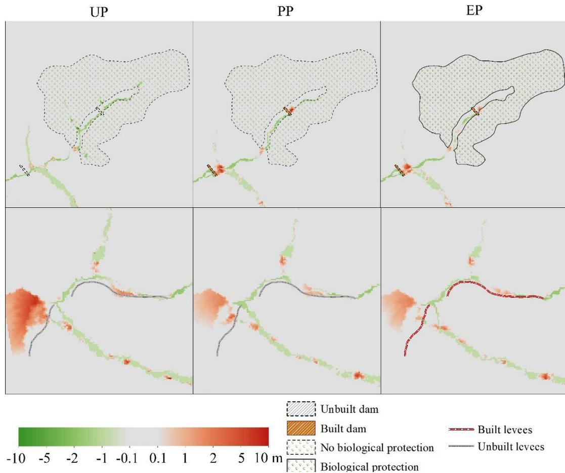
Figure 5. Geomorphic changes at the conclusion of the simulation at key spots for the UP, PP, and EP scenarios. Top row is the upriver section containing dam 1, dam 2 and the vegetation revetment. The bottom row is the downriver section containing levees.
