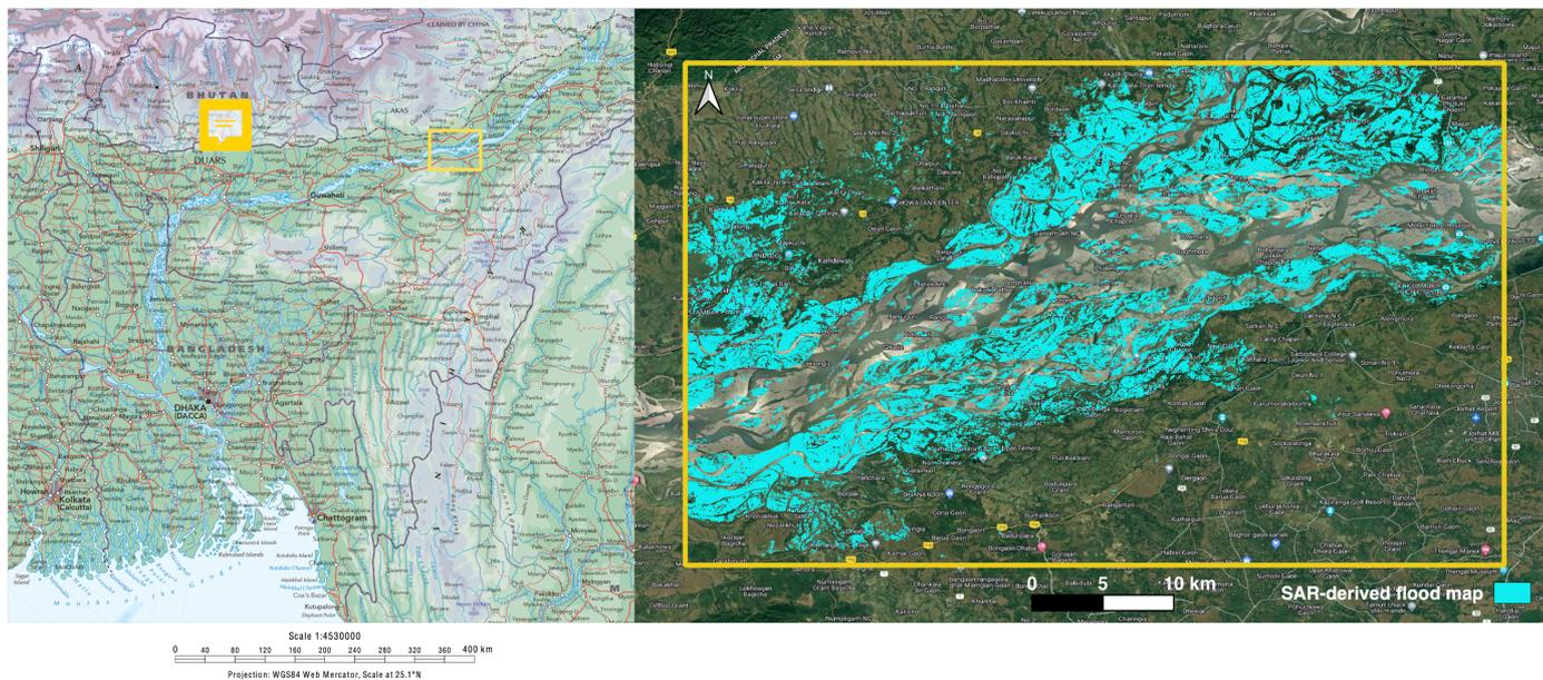
**Figure 2.** Left panel: domain location on the Brahmaputra River in the Assam region of India. Domain size is 57.5 km by 39.3 km. Right panel: Sentinel-1 SAR-derived flood map for the domain of interest. Base map from © Google Maps.
