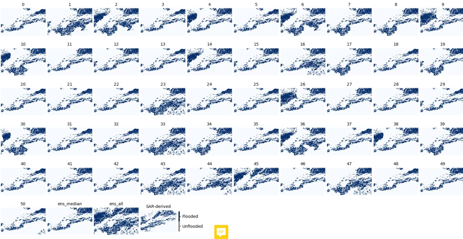
**Figure 4.** Brahmaputra River, Assam region, August 2017. 51 ensemble member forecast flood maps (labelled 0 to 50), *ens<sub>median</sub>* and *ens<sub>all</sub>* all at 1-day lead time and the Sentinel-1 SAR-derived flood map.
