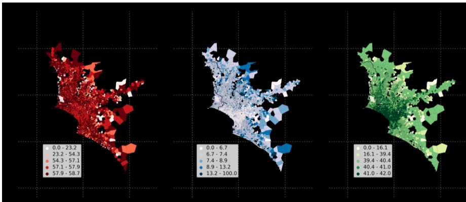
Figure 5. Spatial distribution of the percentage of the main structural material of the residential buildings in Metropolitan Lima in each CVT geocell using the dataset of Gómez Zapata et al., (2021b). The colour scale represents the material type (red: masonry and earthen; blue: reinforced concrete and UNK; green: wooden types). Only CVT that intersected the census-based blocks (INEI, 2017) are shown.
