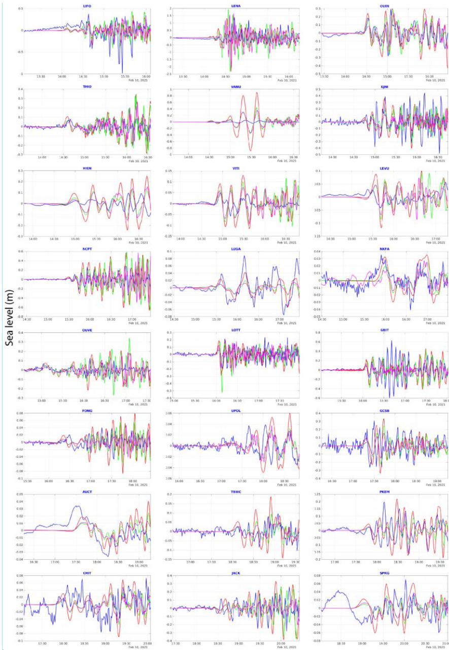
Figure 9: Simulation results obtained with 3 different seismic source model compared to 24 coastal gauge records: uniform slip model (red); non-uniform slip model from waveform inversion (green); USGS finite fault model (magenta); real filtered records (blue).
