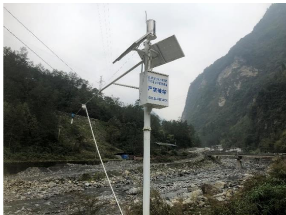
(b) debris flow pre-warning device
