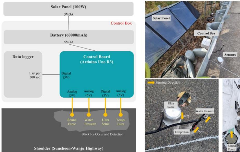
325 **Figure 4:** Configuration and installation photo of multi-sensor for black ice detection. The sensing part of the round force and water pressure sensor faces upward, and the sensing part of the ultrasonic and temperature/humidity sensor faces downward.
