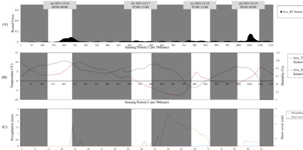
770 **Figure 13:** Data analysis result of temperature/humidity sensor. Round force, temperature/humidity, precipitation, and snow cover were compared.
