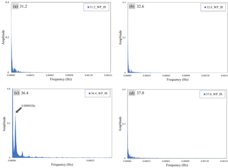
730 **Figure 12:** Fast Fourier transform the result of the data signal of the water pressure sensor. (a), (b), and (d) indicate points where the system dynamics model predicted that black ice would occur, and no waveforms of a particular period were observed. (c) indicates the point where the system dynamics model predicted that black ice did not occur, and a waveform of a particular period was observed.
