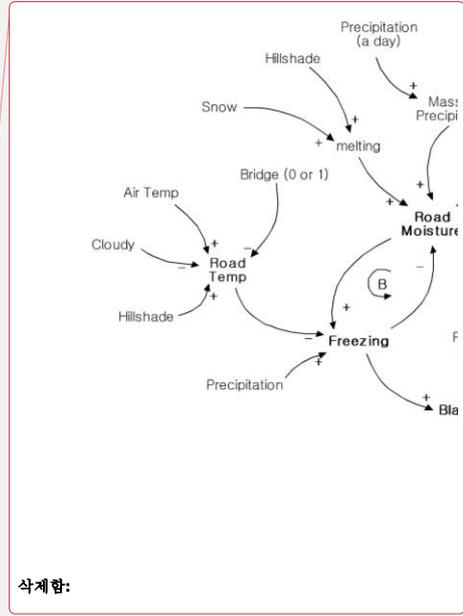
Figure 2: Causal loop of system dynamics model. A causal loop is constructed according to the causal relationship of each factor, and the main results are Road Temperature, Road Moisture, and Black Ice. [+] means proportional, and [-] means inverse proportion.
