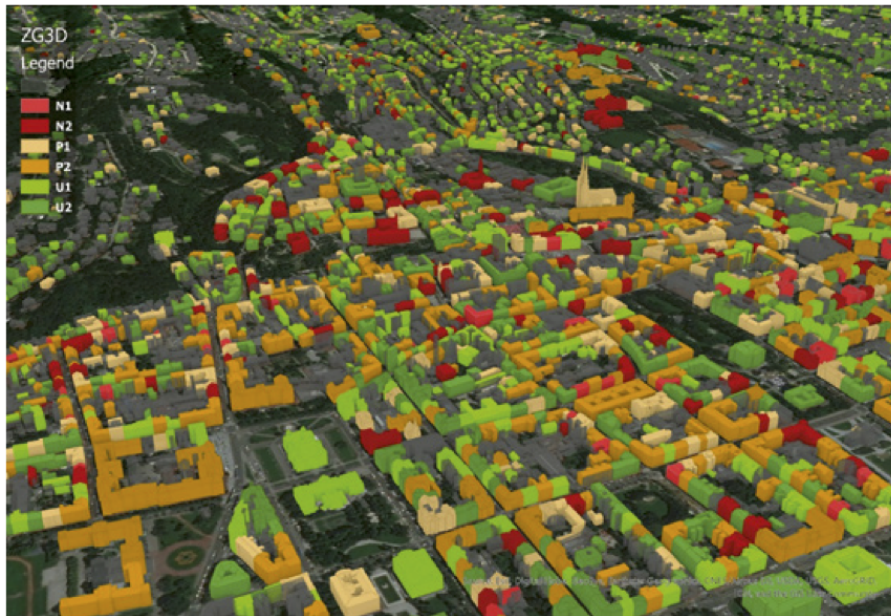
Figure 5. Building damage grades in the city of Zagreb following the 2020 March earthquake
