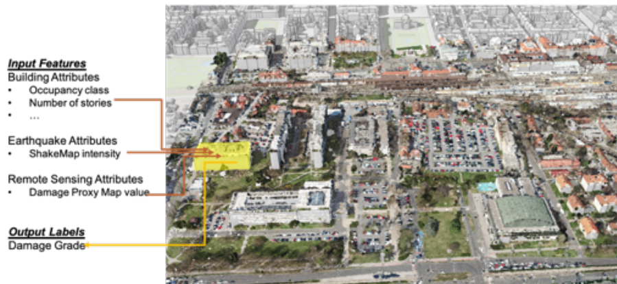
Figure 4. Illustration of the input feature vector and output label vector for a selected building in Zagreb (Map source: Office for Strategic Planning and City Development, Grad Zagreb. URL: https://zagreb.gdi.net/zg3d/ )
