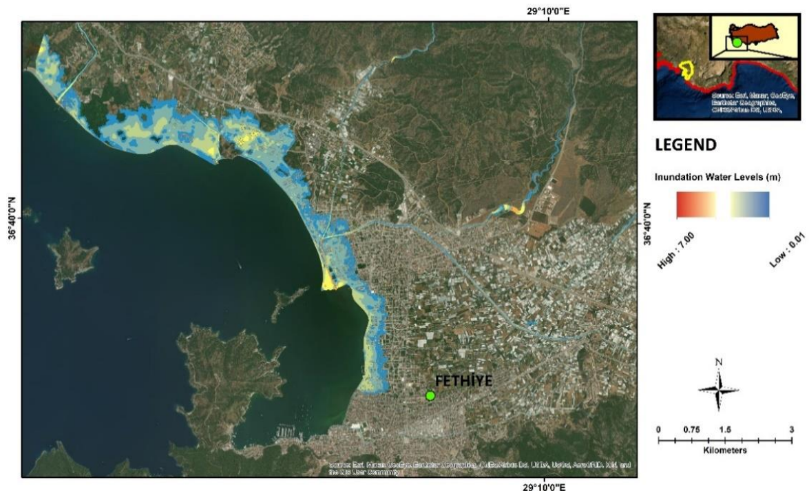
Figure 11. Inundation levels resulted from an earthquake-triggered tsunami hazard (Source: Esri, Maxar, GeoEye, Earthstar Geographics, CNES/Airbus DS, USDA, USGS, AeroGRID, IGN, and the GIS User Community).
