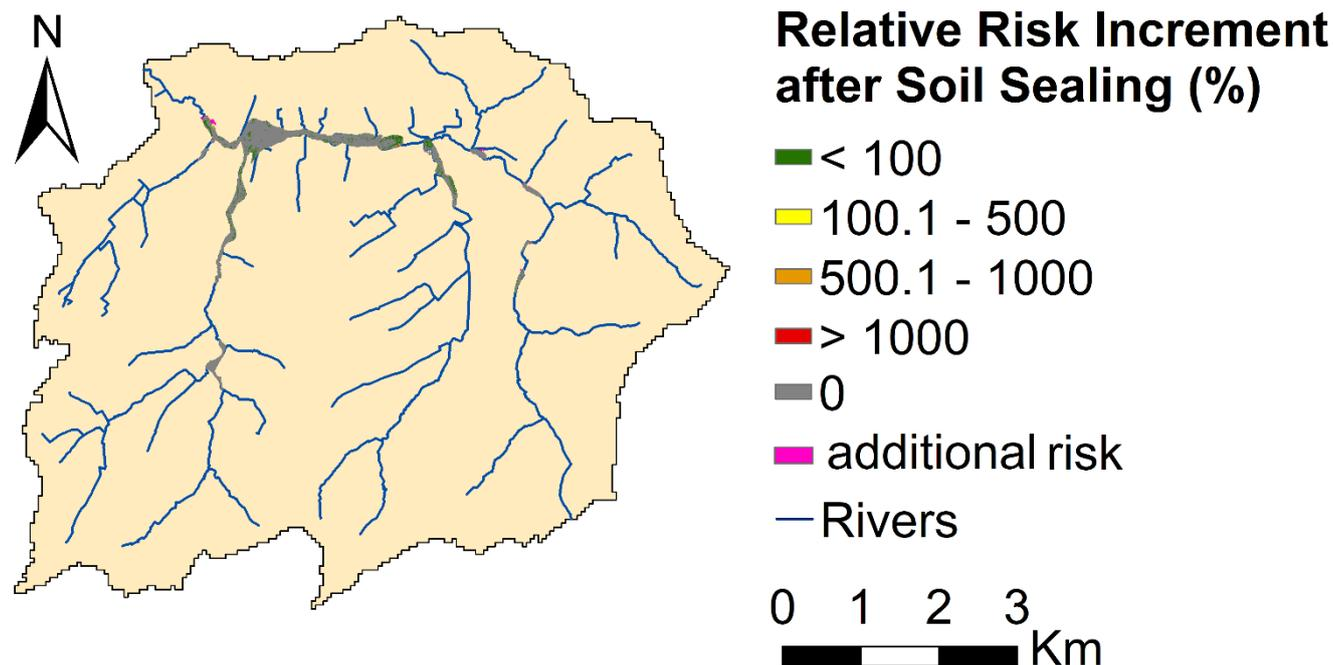
**Figure 10: Relative flood risk increment (%) in the flooded areas in the Maarkebeek catchment after sealing the 750 highest ranked pixels in this land use change scenario. New areas being flooded after soil sealing are depicted as 'additional risk'.**
