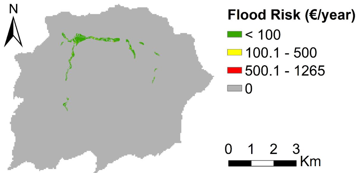
270 **Figure 7:** Flood risk, expressed as expected annual damages (€/year) in each pixel (5m X 5m resolution), in the Maarkebeek catchment based on the four observed flood events. Flood risk is highly localized and highest (€ 1265/year or € 50.6/year/m<sup>2</sup>) in only a few, built-up pixels which were repeatedly flooded. The total flood risk derived from the four flood events in the Maarkebeek catchment equals € 178 252/year.
