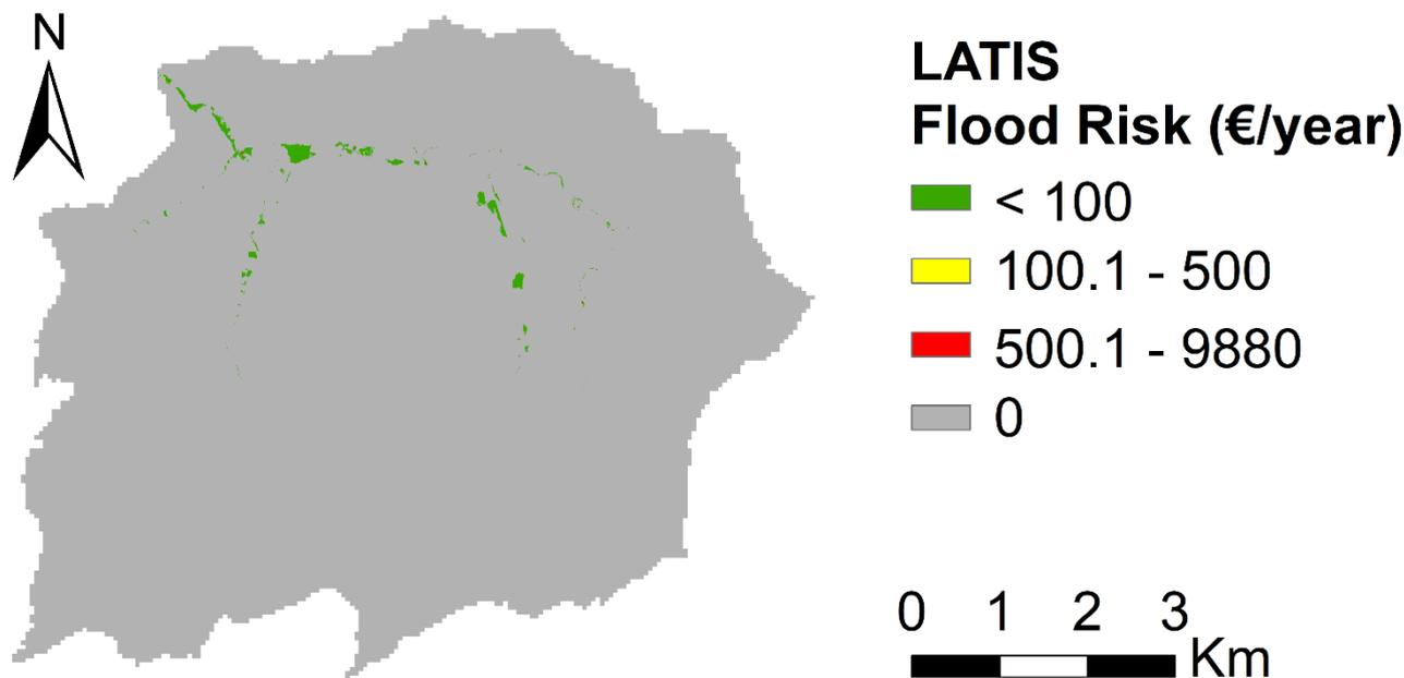
**Figure 11: Flood risk (€/year per pixel of 25 m<sup>2</sup>) in the Maarkebeek catchment as calculated by the LATIS tool based on the flood damages determined for flood events with a return period of 10, 100 and 1000 years (adapted from (VMM, 2015)). (source: Vlaamse Milieumaatschappij, Waterbouwkundig Laboratorium, Maritieme Dienstverlening & Kust, & De Vlaamse Waterweg nv, 2020).**
