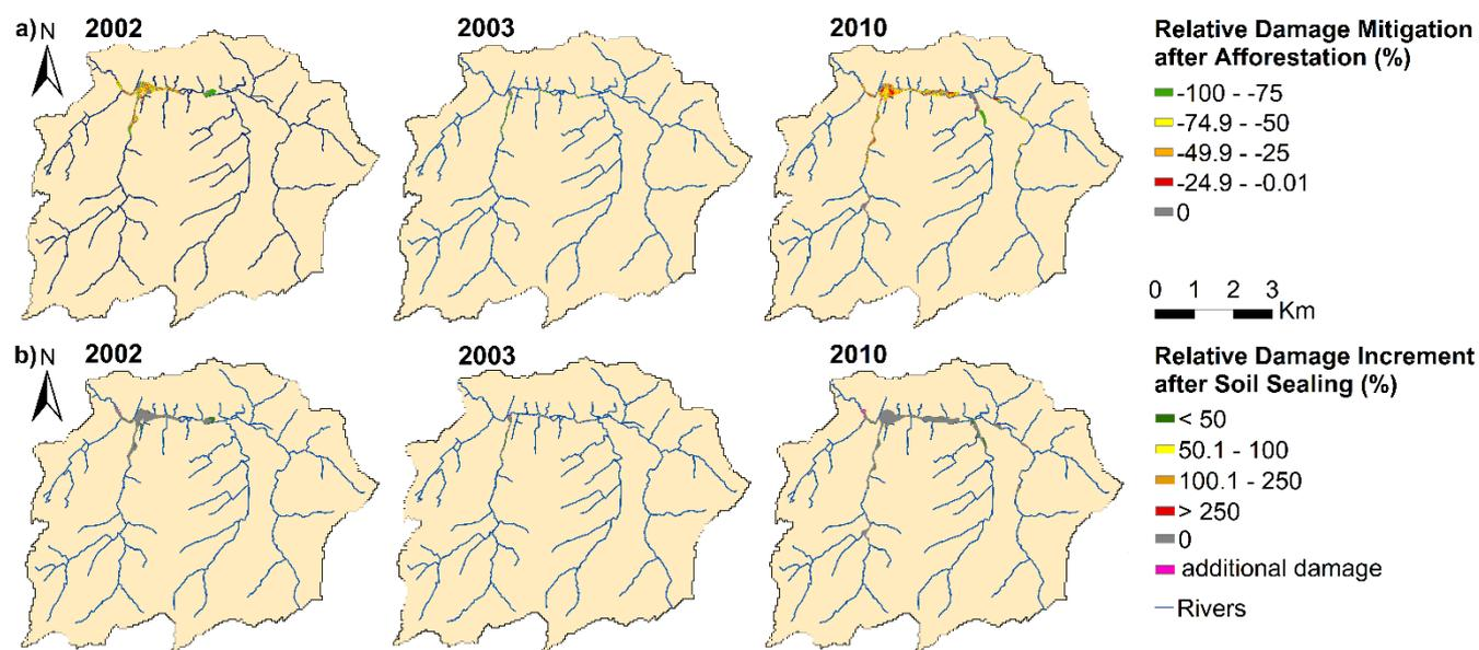
290 **Figure 8: The relative impact in flood damages (%) after (a) implementing the afforestation scenario, resulting in a relative damage mitigation, and after (b) implementing the soil sealing scenario, resulting in a relative flood damage increment. New areas being flooded after soil sealing are depicted as ‘additional damage’, though these areas are limited to a few pixels bordering the river or existing flood extents.**
