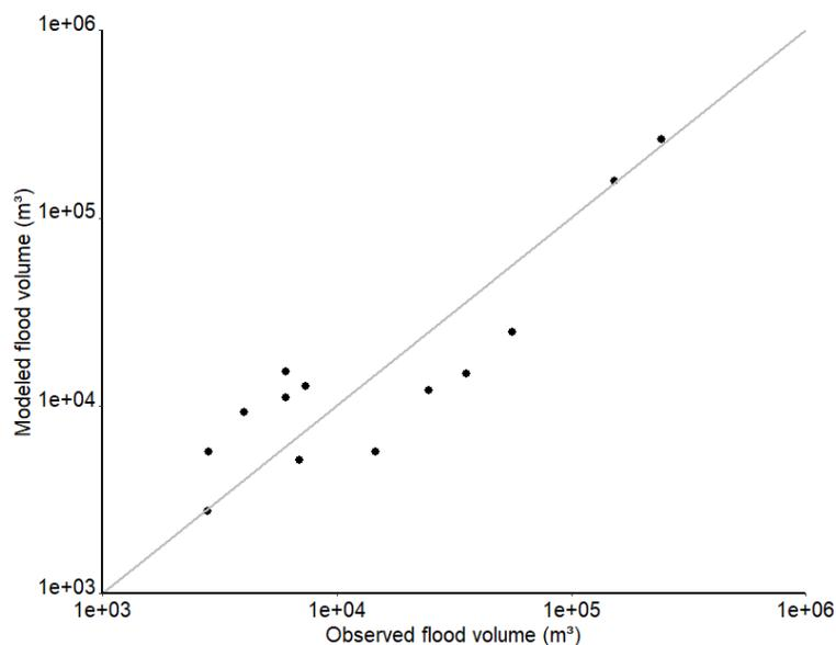
**Figure 5: Scatterplot of the flood volumes derived from the observed flood extents (Observed flood volume,  $m^3$ ) and the flood volumes as modeled by Eq. (6) (Modeled flood volume,  $m^3$ ), with an adjusted  $R^2$  of 0.76 and a relative RMSE of 0.3.**
