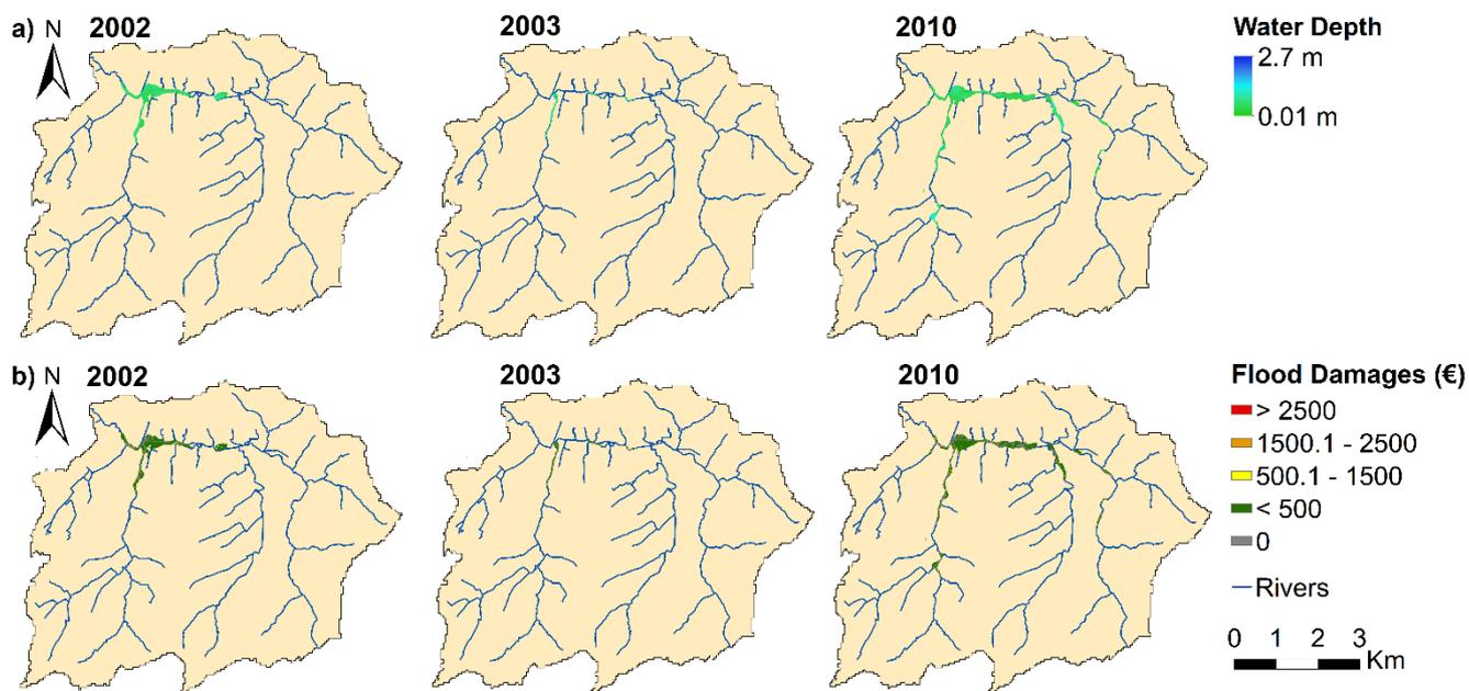
265 **Figure 6:** (a) The inundation depth (m) and (b) the corresponding flood damage (€) per pixel (5m X 5m resolution) derived from the flood damage model in the Maarkebeek catchment resulting from the observed flood events. The total flood damage was respectively € 566 667, € 27 515, € 139 650 and € 1 556 355 for the flood events in February 2002, in August 2002, in January 2003 and in November 2010.
