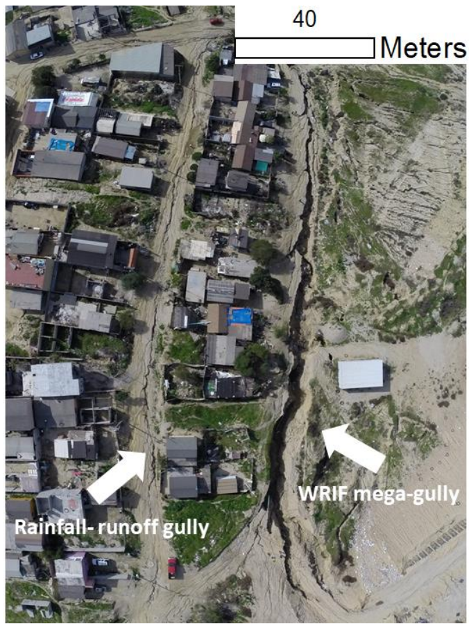
330 Figure 7. High-resolution photograph showing the contrast between gullies generated by rainfall-runoff only (road on left) and mega-gully B (road on right).
