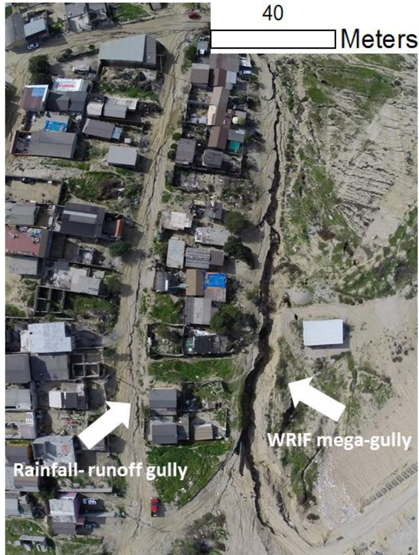
Figure 7. High-resolution photograph showing the contrast between rainfall-runoff and WRIF gullies in the study area.
