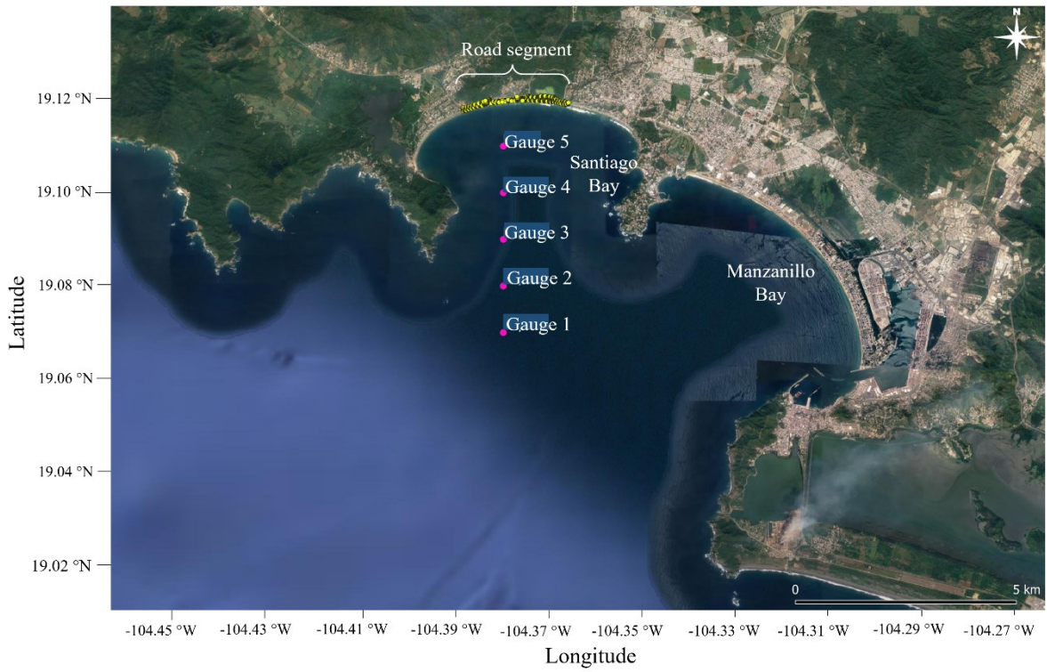
Figure 24: Location of gauges used to obtain the free sea surface elevations and speeds in the simulation. (© Google Earth).
