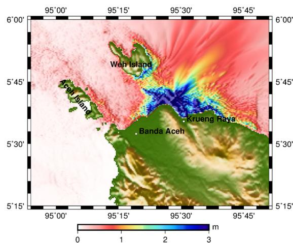
Figure S.4 Maximum tsunami wave amplitude from the corresponding source in Fig. S.3.
