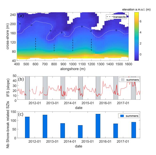
Figure 3. (a) Example of a digital elevation model of Truc Vert beach on 29-Apr-2013, with the colorbar showing elevation amsl. The four cross-shore transects used to compute the inverse beach slope IFS between 1 m and 3 m amsl are indicated by the dashed black lines. (b) Time series of IFS and (c) summer shore-break related injuries.
